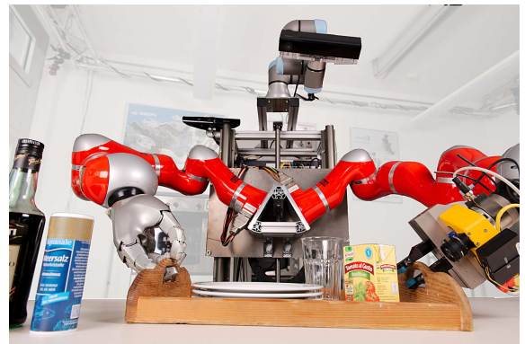
Figure 26: Mobile manipulation platform Boxy available for EASE from the beginning of the project.
