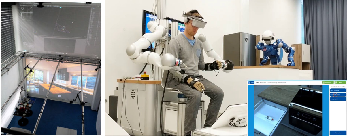
Figure 1.66: The EASE BASE laboratory for recording human everyday activities (left) and the experimental kitchen setup at EASE partner DLR with the autonomous mobile manipulation platform MobileJustin .
