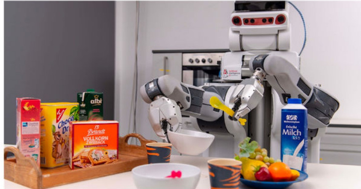
A PR2 robot sets a table during a demonstration of cognitively-enabled robot manipulation using CRAM. Image courtesy of the EASE interdisciplinary research center at the University of Bremen, Germany.
